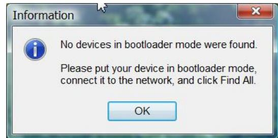
The bootloader window outlines the firmware update process in three easy steps. The first step advises that the 525N must, itself, be in the 'bootloader' (firmware update) mode.
